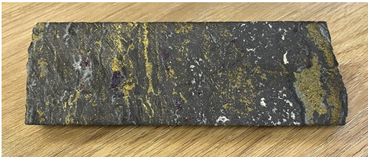
Figure 2: Drill core from previously released diamond drill hole WD22-01 from approximately 544m (1,785ft) downhole from the 'Goldilocks Zone' which assayed 94.5g/t In, 2.8% Cu, 0.49g/t Au, 39.5g/t Ag.
